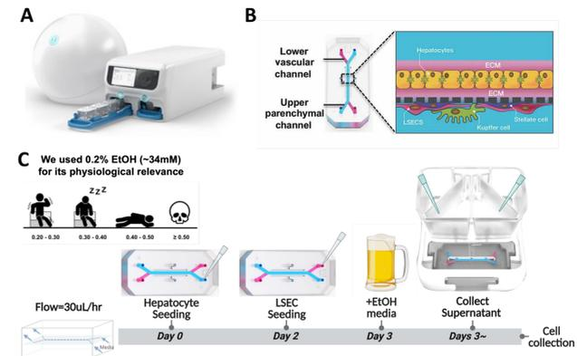
Figure 1. Flowchart of our human Liver-on-a-Chip experiments. (A) Image of organ-on-a-chip culture instruments. (B) Schematic image of human Liver-on-a-Chip. (C) The experiment protocol was used in this study.
